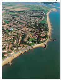
direction. The works at Cobbolds Point have created conditions which are more capable of retaining material under a range of conditions. However, this has also resulted in a readjustment of the material within the artificial bays created causing a draw down on beaches central to each bay against the back shore defences.
