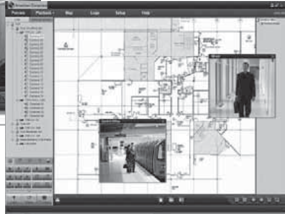
Remote Client - Electronic Maps (add camera icons, monitor alarms)
