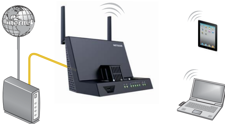
Figure 5. Smart Cradle using an Ethernet WAN Internet connection
