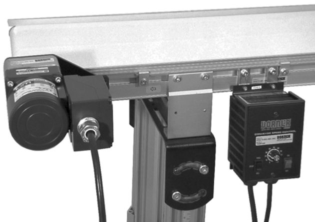
Typical Variable Speed Mounting on Conveyor
