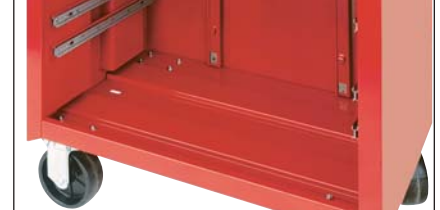
"C"-Channel Base - Double "C"-Channel reinforcement on inside of bottom on roller cabinets increases load bearing capacity by over 30%. "C"-Channel also keeps box rigid and square.
