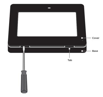
Figure 1: Removing the Cover
