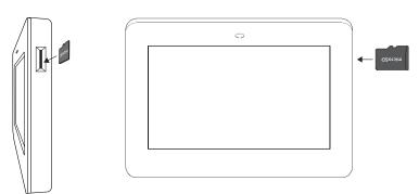
Figure 11: Inserting a microSD Card
