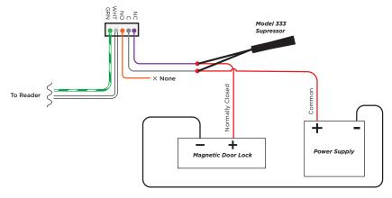
Figure 4: Typical Magnetic Lock Wiring
