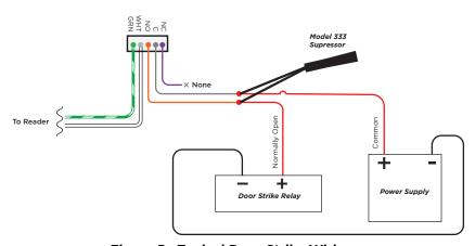
Figure 5: Typical Door Strike Wiring
