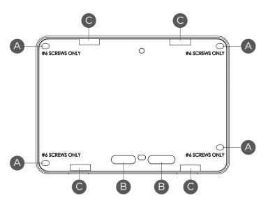
Figure 2: Mounting Hole Locations
