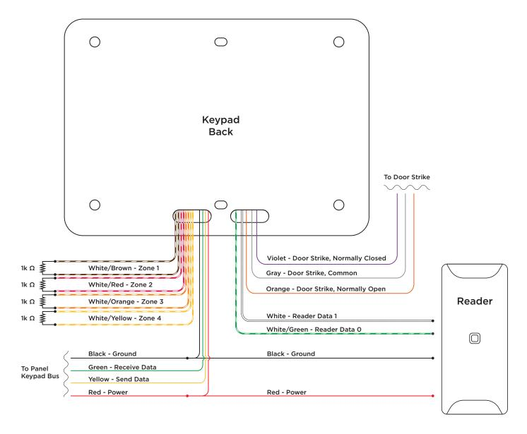
Figure 3: Keypad Wiring
