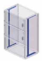
Installation of uprights on a 2 compartments enclosure with integrated plinth
