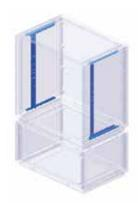
Installation of uprights on a cabinet complete with plinth (not integrated)
