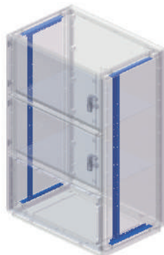
Installation of uprights on a 2 compartments enclosure with integrated plinth
