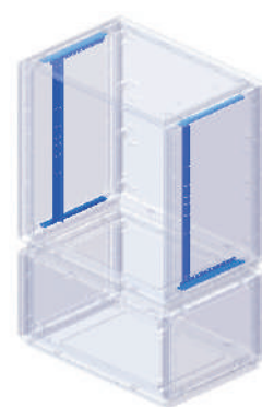
Installation of uprights on a cabinet complete with plinth (not integrated)
