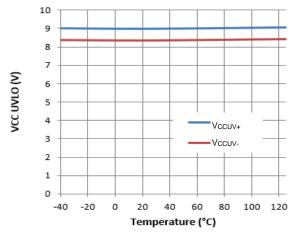
Figure 26. VCC UVLO vs. Temperature
