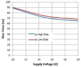
Figure 8. Rise Time vs. Supply Voltage
