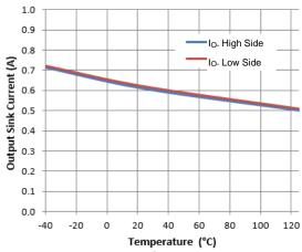
Figure 19. Output Sink Current vs. Temperature
