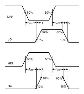
Figure 2. Switching Time Waveform Definitions
