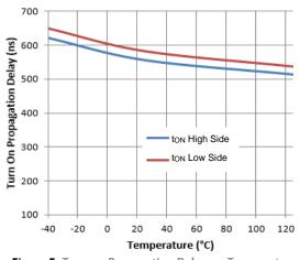
Figure 5. Turn-on Propagation Delay vs. Temperature
