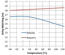
Figure 15. Delay Matching vs. Temperature
