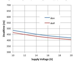
Figure 24. Deadtime vs. Supply Voltage
