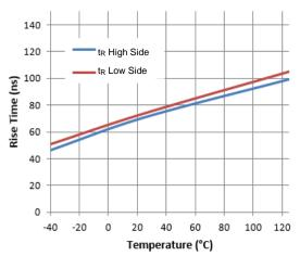
Figure 9. Rise Time vs. Temperature
