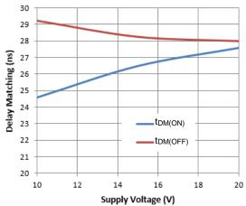
Figure 14. Delay Matching vs. Supply Voltage
