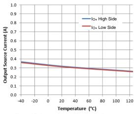
Figure 17. Output Source Current vs. Temperature
