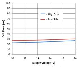
Figure 10. Fall Time vs. Supply Voltage
