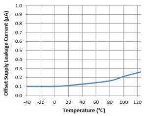
Figure 27. Offset Supply Leakage Current vs. Temperature
