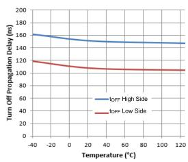
Figure 7. Turn-off Propagation Delay vs. Temperature
