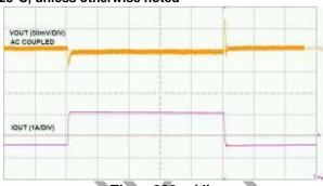
Time- 200μs/div Load Transient Test I<sub>ουτ</sub>=1.5A to 3A. Step at 0.8A/μs
