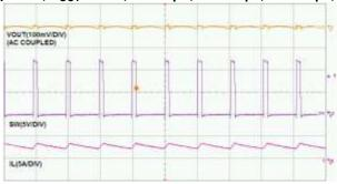
Time- 2µs/div Steady State Test I<sub>OUT</sub> =3A
