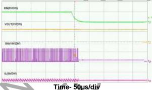
Shutdown Through Enable (No Load)
