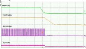
Time- 50µs/div Shutdown Through Enable (I<sub>OUT</sub> =1A)
