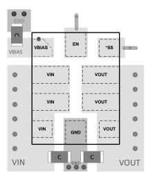
\* SS pin trace must be less than 0.01 inch for SS = Float configuration.
