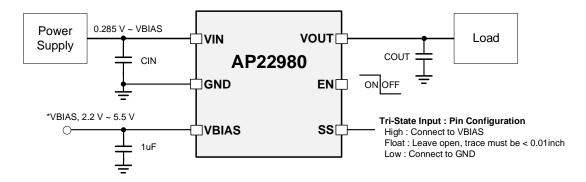
$^{\ast}$  If V\_{IN} is higher than 2.2V then VBIAS pin can be connected to VIN.
