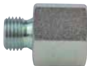
B.21.0089 Nipples 1/4" bsp female - 7/16" unf male
