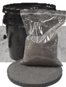
Bit Sharpening Pot Plastic bucket that includes a cast iron plate and #60 aluminum oxide sand for sharpening dull core bits. The sand acts as an abrasive to expose the diamonds in the segments.
