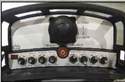
Radio remote control has a range of 300 feet for safety and convenience
