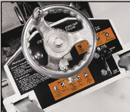
Dial screw feed raise and lower handle with comprehensive saw operation control panel.
