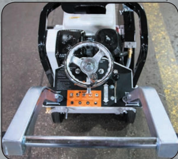
Dial screw feed raise and lower handle with comprehensive saw operation control panel.
