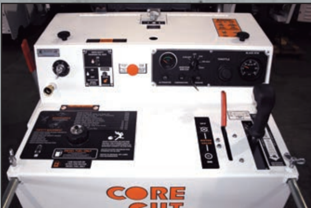
Mini- Groover control panel with power raise and lower controls, drive control and gauge
