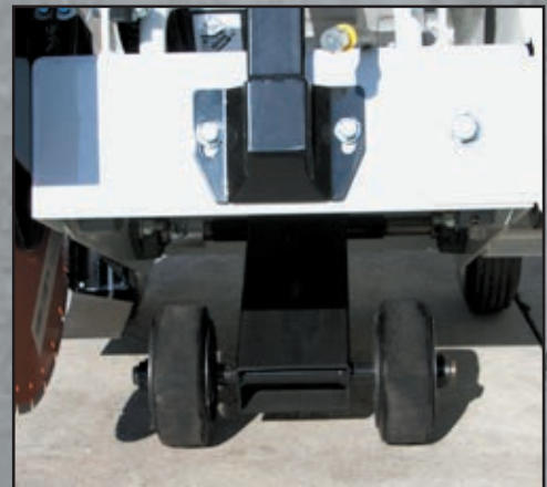
Heavy duty boxed raise/lower wheel shaft
