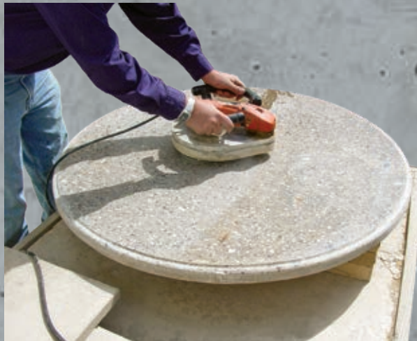
One of three 5" grinding platens (Velcro® surface)
