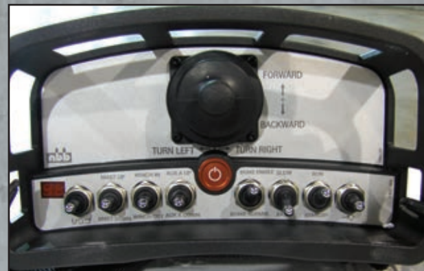
Radio remote control has a range of 300 feet for safety and convenience
