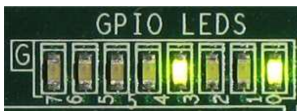
Figure 11 LED Status when running Sending Demo with Non-Jumbo frame
