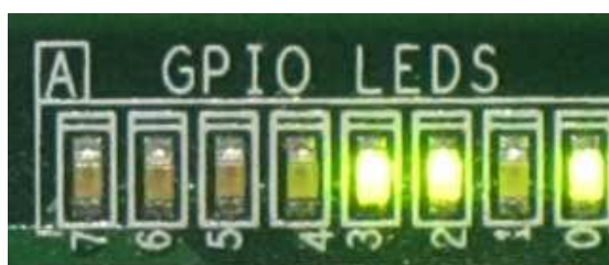
Figure 13 LED Status when running Sending Demo with Jumbo frame
