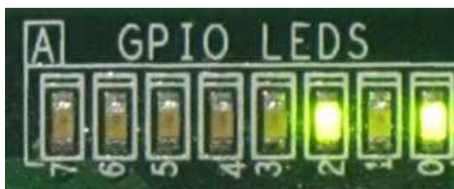
Figure 9 LED Status after push StartSW when DIPSW[1]=ON
