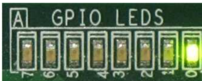
Figure 8 LED Status after push StartSW when DIPSW[1]=OFF
