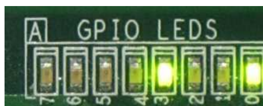
Figure 11 LED Status when running Sending Demo with Non-Jumbo frame
