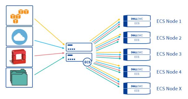
Figure 4. Active/Passive HA Kemp ECS Connection Manager servicing the ECS cluster
