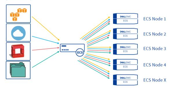
Figure 3. Single Kemp ECS Connection Manager servicing the ECS cluster
