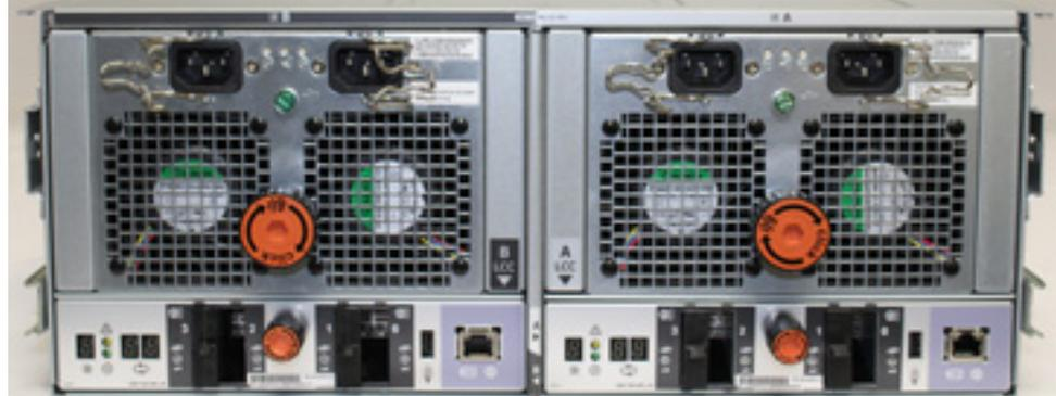
Each controller has 4 SAS ports (laid out as 2 pairs). Standard Data Domain systems, and systems with the licensed HA feature only use ports 0 and 2 on each controller. Ports 1 and 3 typically have a plastic plug blocking the unused ports to make inserting a cable into the correct ports easier.
