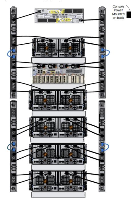
Figure 35 Recommended single phase power connections for DD9800
