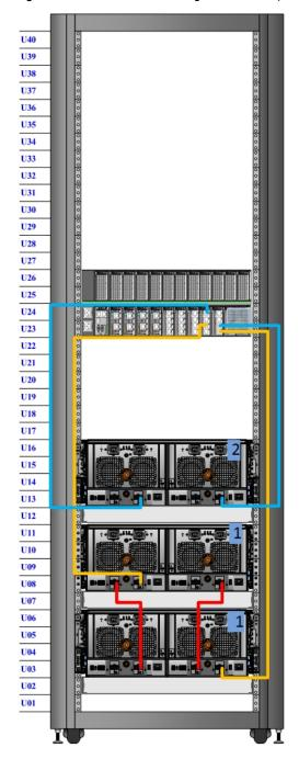
Figure 14 Recommended cabling for DD7200 (3TB drives)
