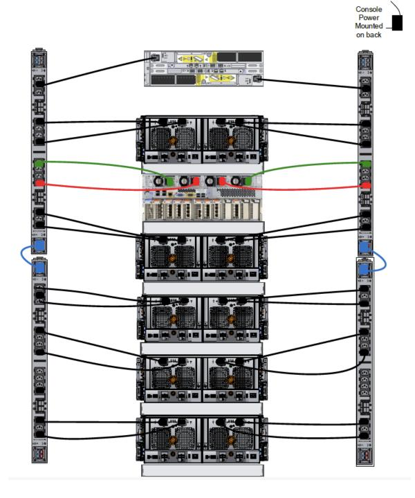
Figure 43 Recommended 3-phase delta power connections for DD9800
