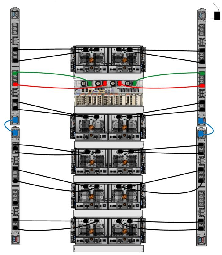
Figure 42 Recommended 3-phase delta power connections for DD9500 system
