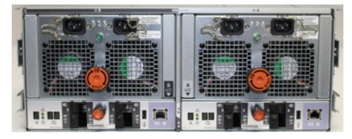
Each controller has 4 SAS ports (laid out as 2 pairs). Standard Data Domain systems, and systems with the licensed HA feature only use ports 0 and 2 on each controller. Ports 1 and 3 typically have a plastic plug blocking the unused ports to make inserting a cable into the correct ports easier.
