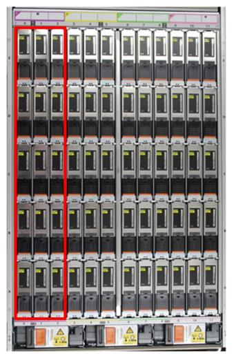
The next table shows how the drives are distributed by packs (groups) and numbered physically. The bottom of the table represents the front of the shelf
