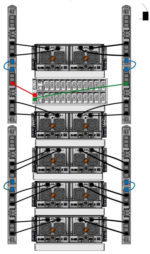
**Figure 32** Recommended single phase power connections for the DD4200, DD4500, and DD7200 systems
