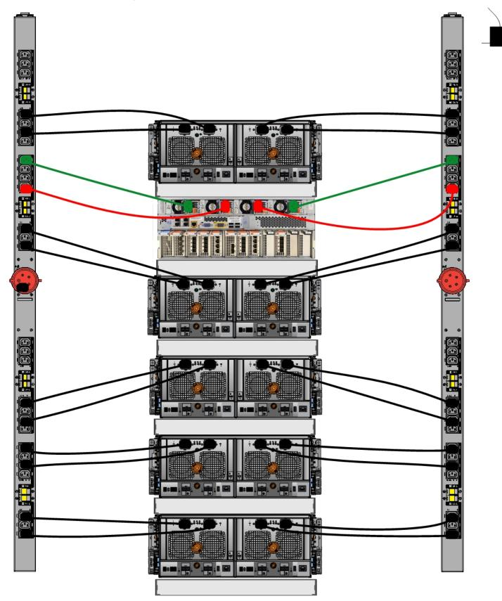
Figure 49 Recommended 3-phase wye power connections for DD9500 system
