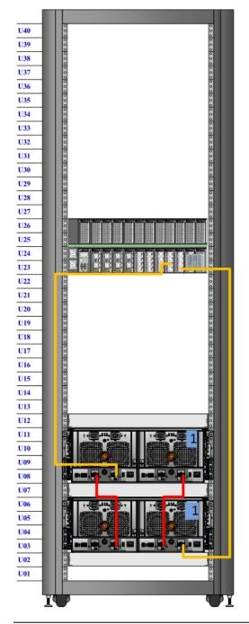
Figure 7 Recommended cabling for DD4200 (3TB drives)
