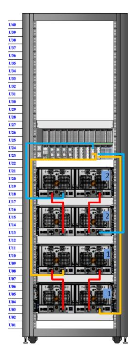
Figure 17 Recommended cabling for DD7200 with DD Cloud Tier
