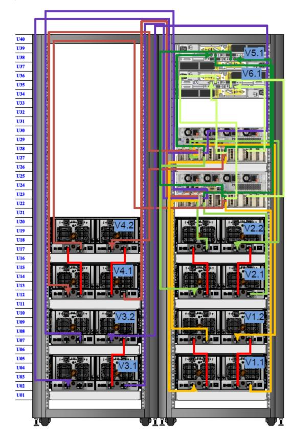
Figure 29 Cabling for HA DD9500 and DD9800 systems with DD Cloud Tier
