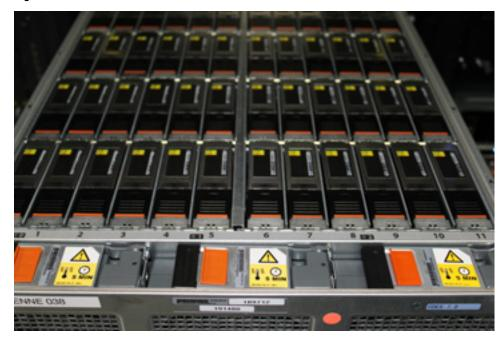
Figure 2 Fans and disk drives inside the disk enclosure
