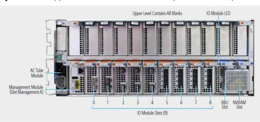
Figure 53 Rear view (systems with Extended Retention software option or DD Cloud Tier)
