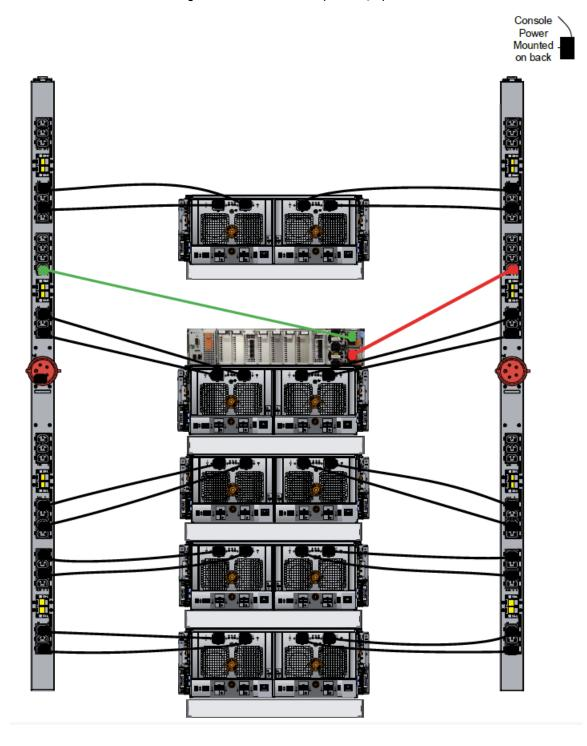
Figure 47 Recommended 3-phase wye power connections for DD9300
