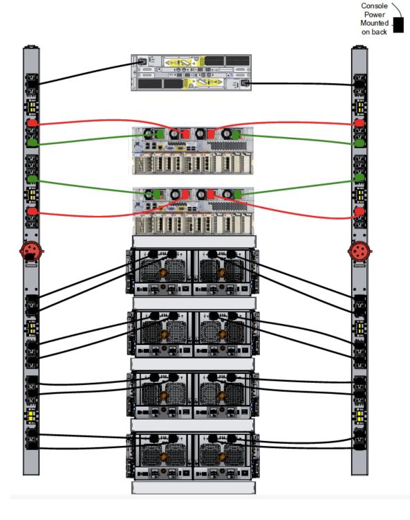
Figure 51 Recommended 3-phase wye power connections for DD9800 with HA
