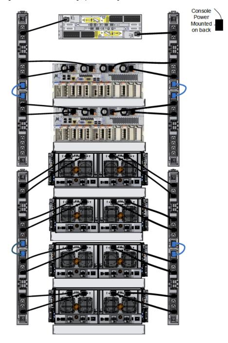
Figure 36 Recommended single phase cabling for DD9800 with HA
