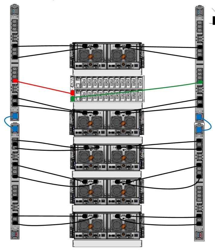
Figure 39 Recommended 3-phase delta power connections for DD4200, DD4500, and DD7200 systems
