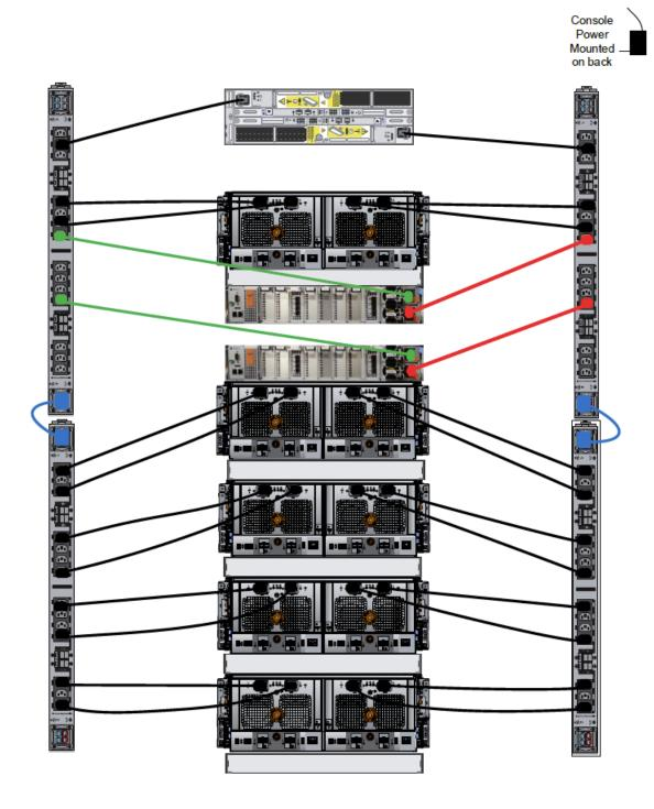
Figure 41 Recommended 3-phase delta power connections for DD9300 with HA
