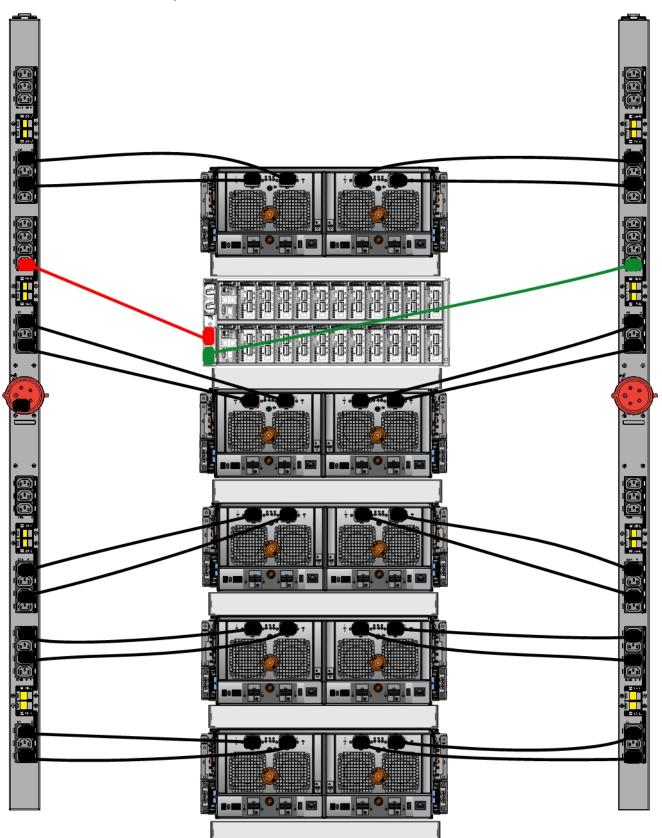
**Figure 46** Recommended 3-phase wye power connections for DD4200, DD4500, and DD7200 systems
