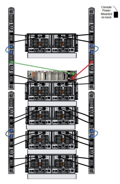
Figure 33 Recommended single phase power connections for the DD9300
