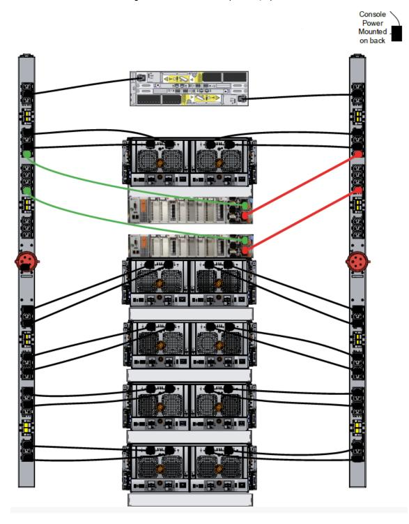
Figure 48 Recommended 3-phase wye power connections for DD9300 with HA
