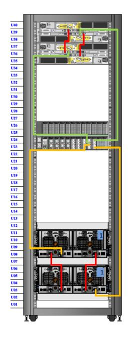
Figure 11 Recommended cabling for DD4500 with DD Cloud Tier
