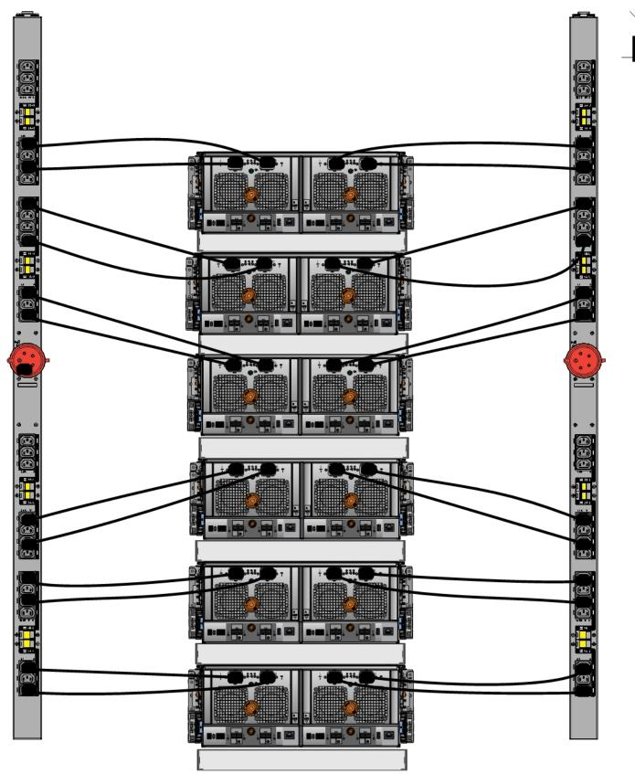
Figure 45 Recommended 3-phase wye power connections for the DS60 expansion shelves (full-racked)
