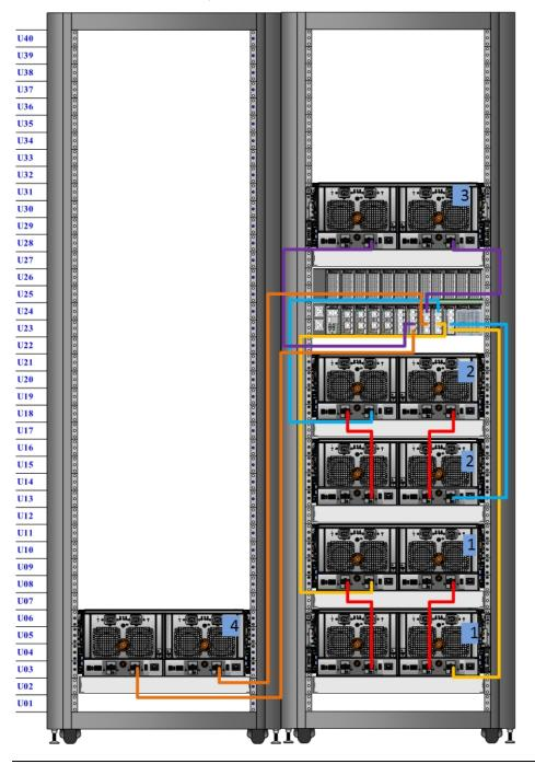
Figure 18 Recommended cabling for DD7200 (4TB drives) with Extended Retention software
