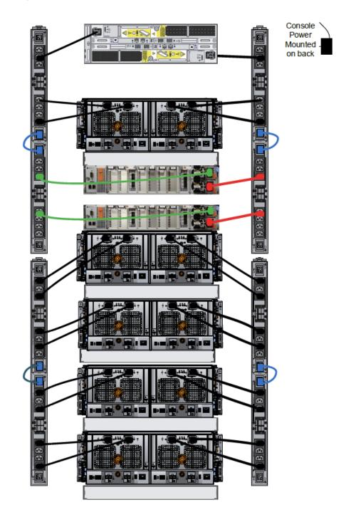
Figure 34 Recommended single phase power connections for DD9300 with HA
