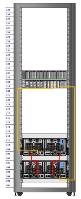
Figure 9 Recommended cabling for DD4500 (3TB drives)
