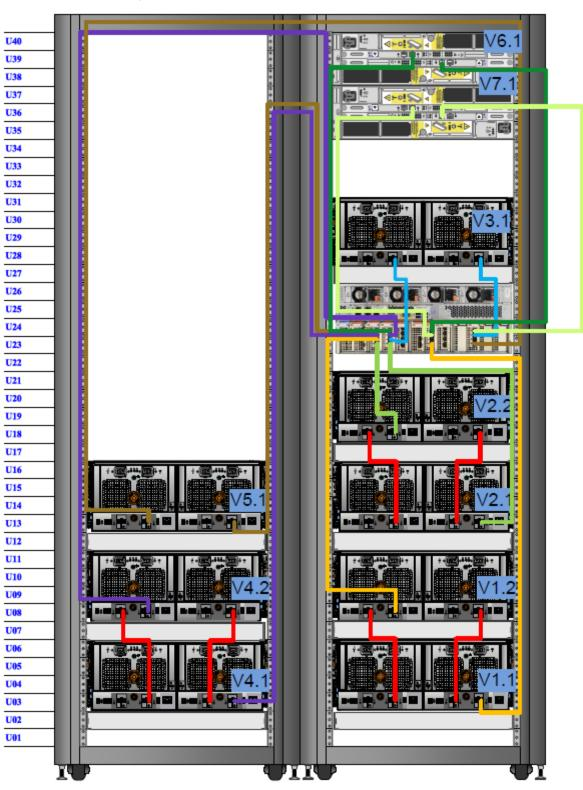
Figure 28 Cabling for DD9500 and DD9800 systems with DD Cloud Tier
