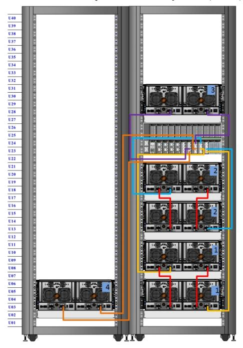
Figure 16 Recommended cabling for DD7200 (3TB drives) with Extended Retention software
