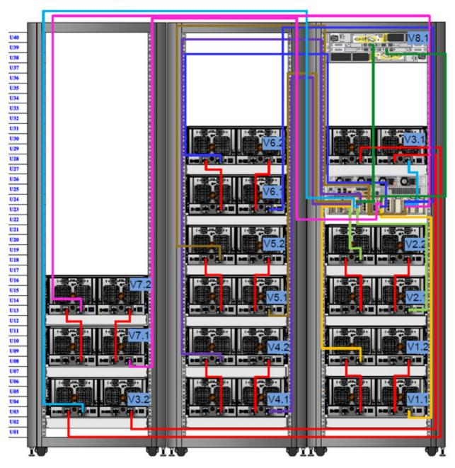
Figure 30 Cabling for DD9500 and DD9800 systems with ERSO
