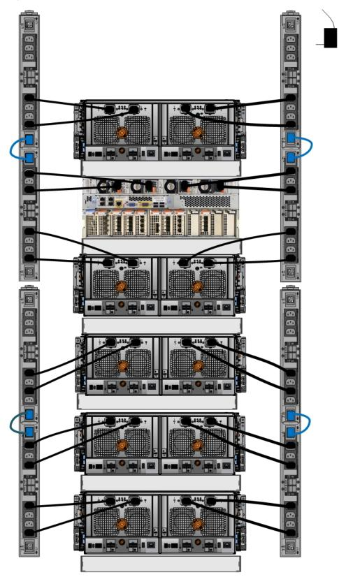
Figure 37 Recommended single phase power connections for the DS60 (full-racked)
