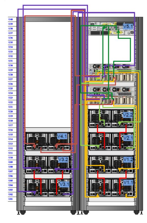
Figure 27 Cabling for HA DD9500 and DD9800systems
