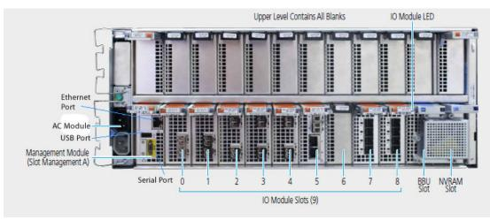
Figure 52 Rear view (systems without Extended Retention software option or DD Cloud Tier)
