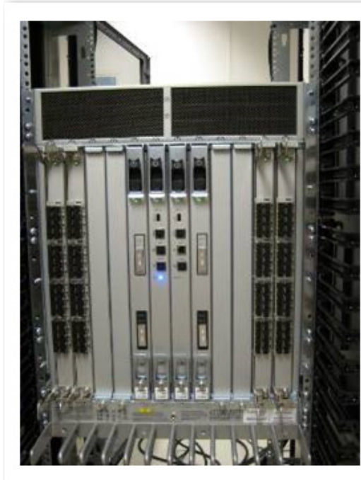
Figure 37 Fully install director - flush against front rails
