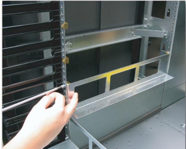
Figure 60 Installing the upper left shelf bracket
