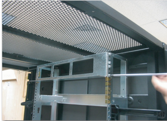
Figure 50 Removing the upper shelf bracket
