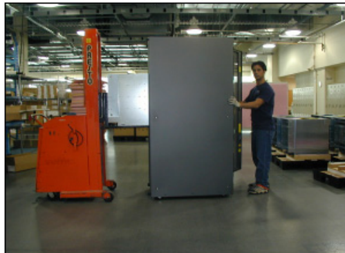
Figure 36 Guiding director onto rails require one person at rear
