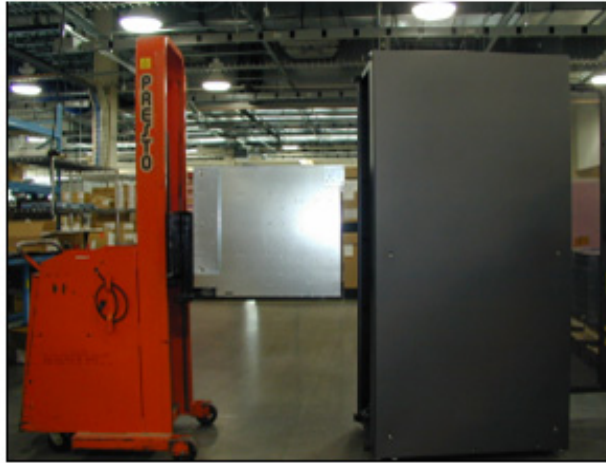
Figure 35 Moving Director unit with power lift
