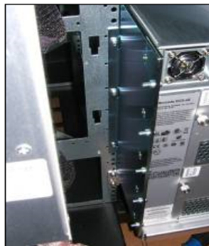
Figure 39 Attaching transportation brackets
