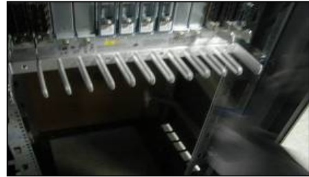
Figure 40 Cable management combs for ED-DCX-B only
