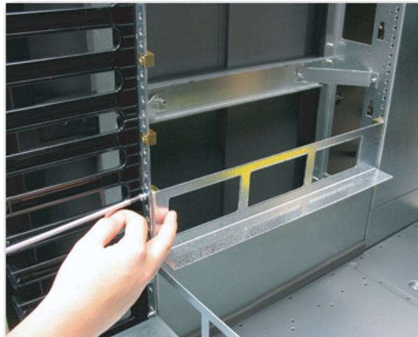
Figure 51 Installing the upper left shelf bracket
