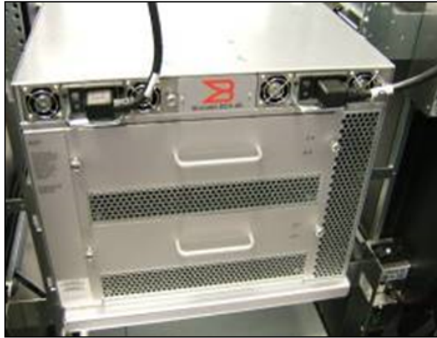
Figure 42 Connectors' positioning for ED-DCX8510-4 and ED-DCX-4S-B
