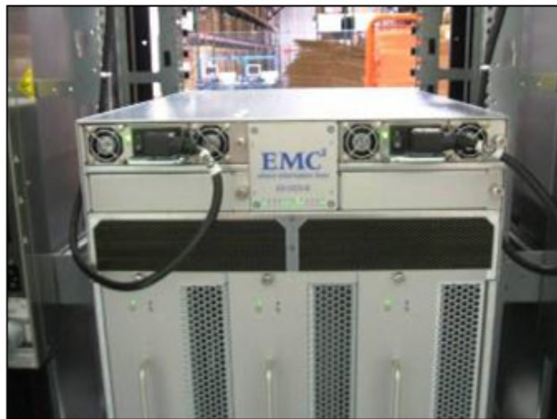
Figure 41 Power cable connection for ED-DCX8510 and ED-DCX-B
