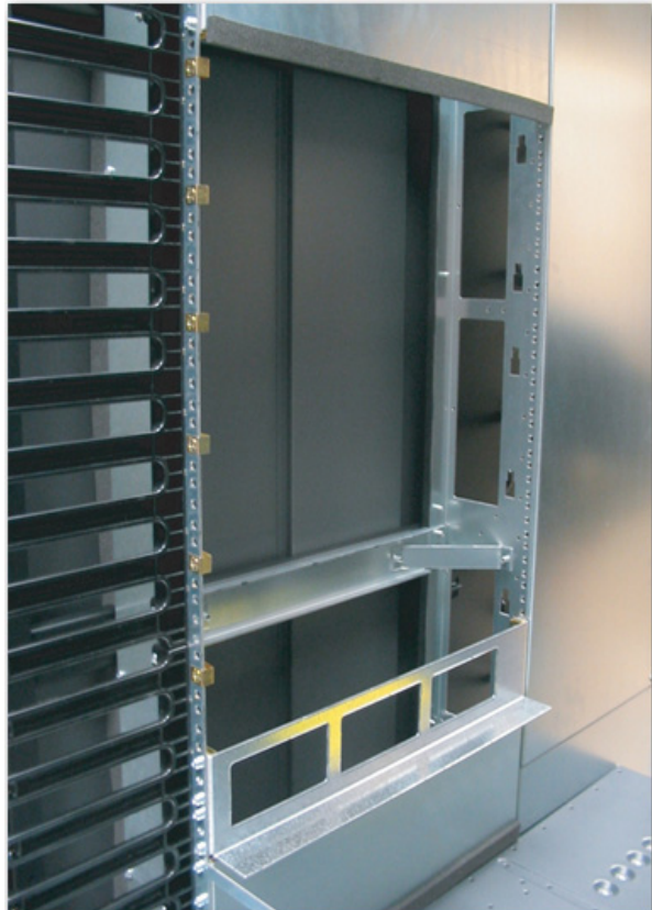
Figure 49 Upper left shelf bracket and clip nuts
