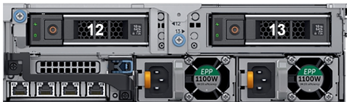
Figure 7 Rear panel hard drives
