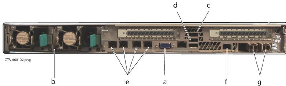
**Figure 4. Rear view of Gen 8 appliance**
