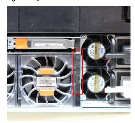
The next photo shows the location of the system LED legend label. Figure 63 on page 119 shows the power supply LEDs. Other front LEDs are shown in Figure 64 on page 120. LED states are described in Table 68 on page 120.
