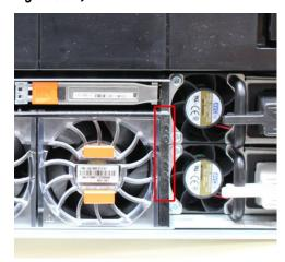
The next photo shows the location of the system LED legend label. Figure 35 on page 63 shows the power supply LEDs. Other front LEDs are shown in Figure 36 on page 64. LED states are described in Table 30 on page 64.
