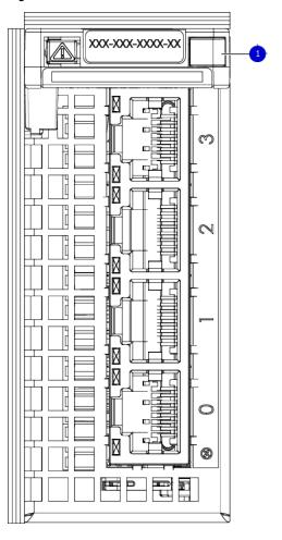
Figure 56 I/O module Power/Service LED location
