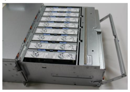
Figure 104 Releasing a memory riser
