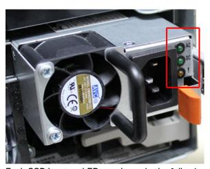
Each SSD has two LEDs as shown in the following figure. The lower left corner of the housing around each fan acts as an LED, glowing amber when the fan has failed.
