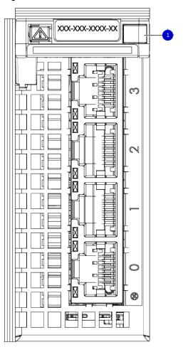
Figure 70 I/O module Power/Service LED location
