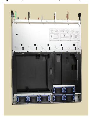
Figure 15 Top view of SP module (system shown)
