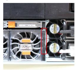
The next photo shows the location of the system LED legend label. Figure 43 on page 77 shows the power supply LEDs. Other front LEDs are shown in Figure 44 on page 78. LED states are described in Table 36 on page 78.
