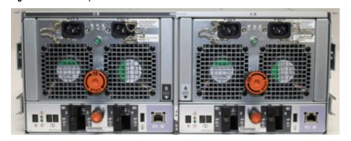
Each controller has 4 SAS ports (laid out as 2 pairs). Standard Data Domain systems, and systems with the licensed HA feature only use ports 0 and 2 on each controller. Ports 1 and 3 typically have a plastic plug blocking the unused ports to make inserting a cable into the correct ports easier.
