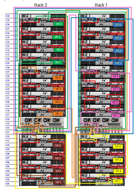
Figure 14 Cabling for HA DD9500/DD9800 systems in two racks
