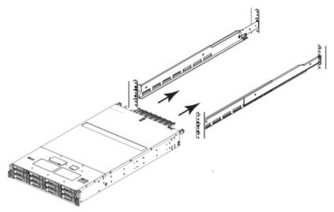
11. Secure the unit to the NEMA channel and rails using four screws, two on each side.
