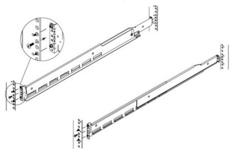
4. Insert one screw into the lower hole to hold the front of the rails in place. Do not fully tighten the screw at this time.
