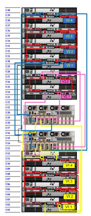
Figure 13 Cabling for HA DD9500/DD9800 systems in one rack
