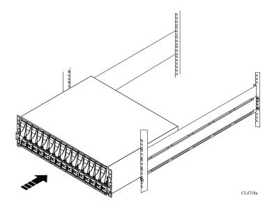
When the enclosure slides to the back of the cabinet, the rear tabs on the rails insert into the two notches in the rear of the enclosure. The tabs secure and support the rear of the enclosure (Figure 9 on page 14).
