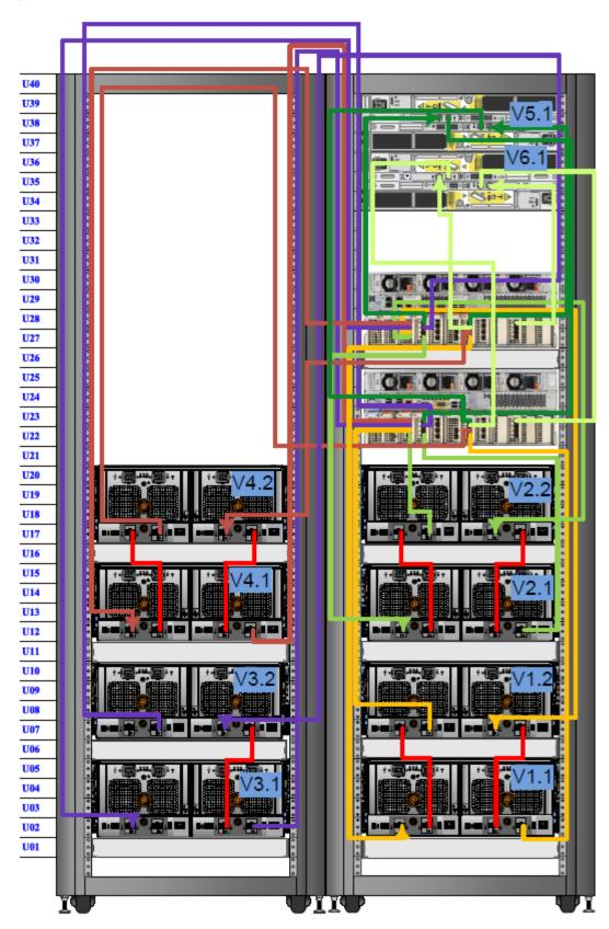
Figure 17 Cabling for HA DD9500 and DD9800 systems with Data Domain Cloud Tier
