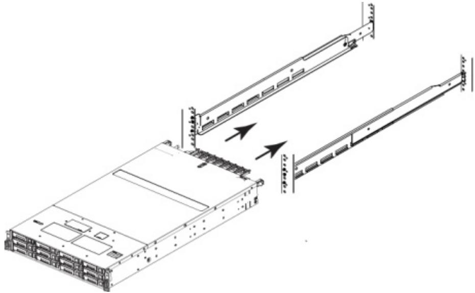
11. Secure the unit to the NEMA channel and rails using four screws, two on each side.
