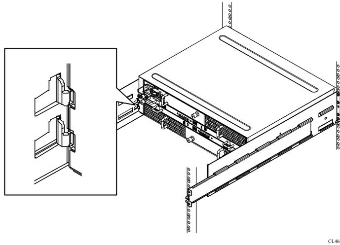
5. Once the enclosure is completely seated into the rear tabs, secure the enclosure, tighten the screws (two on each rail) that secure the rails to the channels.
