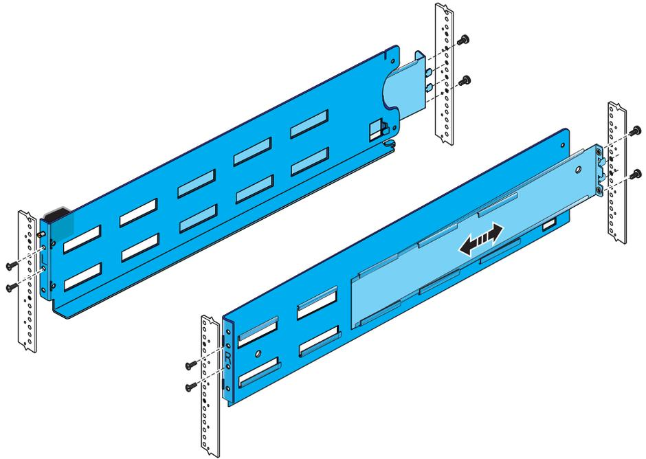
8. Repeat the steps to attach the remaining bracket to the other side of the rack.
