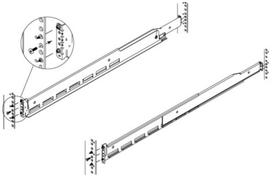
4. Insert one screw into the lower hole to hold the front of the rails in place. Do not fully tighten the screw at this time.
