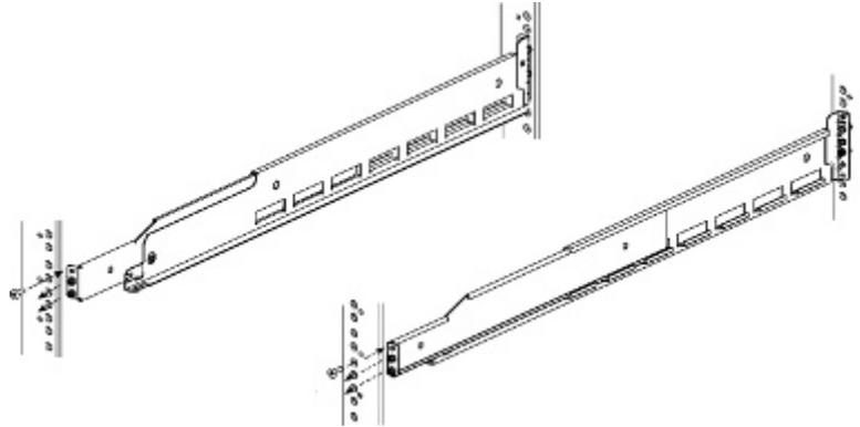
6. Use an 18-inch screwdriver (minimum) to secure the rear of the rail to the NEMA channel using one screw.
