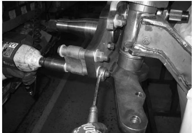
Figure 29. Removal of Brake Bolts and Anchor Pin
