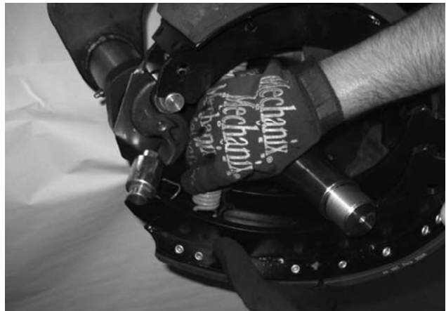
Figure 28. Removal of Return Spring
