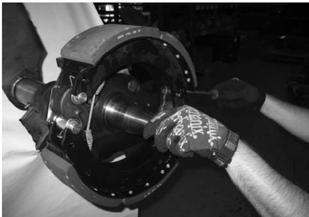
Figure 27. Removal of Outer and Inner Retaining Spring
