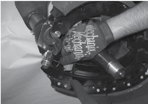
Figure 47. Removal of Return Spring
