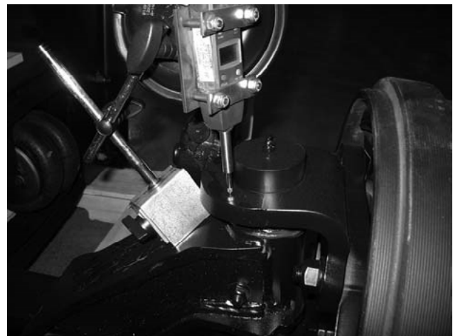
Figure 6 Vertical End Play Checking
