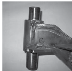
Figure 22. Kingpin After Cleaning
