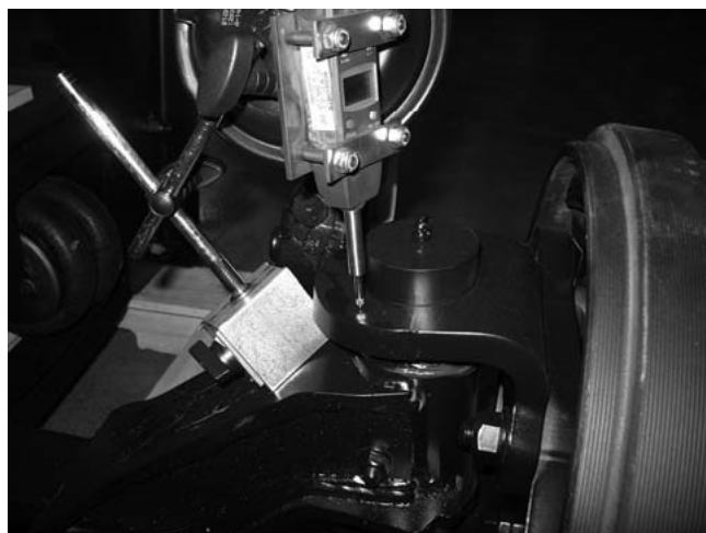
Figure 6 Vertical End Play Checking
