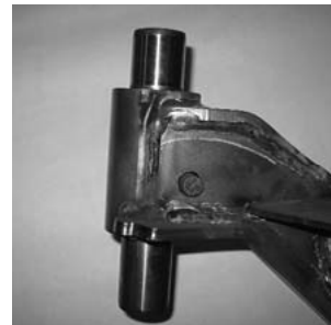
Figure 11. Kingpin After Cleaning
