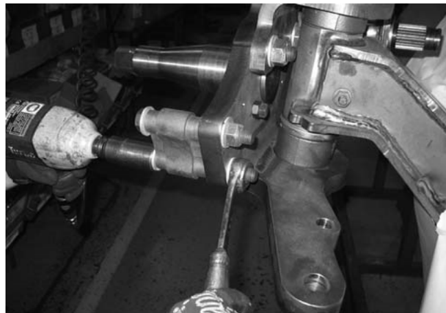
Figure 29. Removal of Brake Bolts and Anchor Pin
