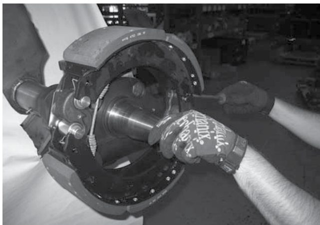
Figure 46. Removal of Outer and Inner Retaining Spring
