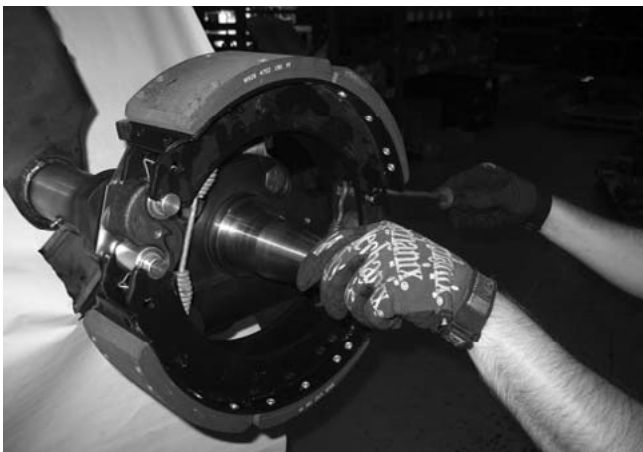
Figure 27. Removal of Outer and Inner Retaining Spring
