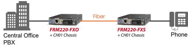
Figure 2 : Voice Transmission from 2km to 120km over fiber
