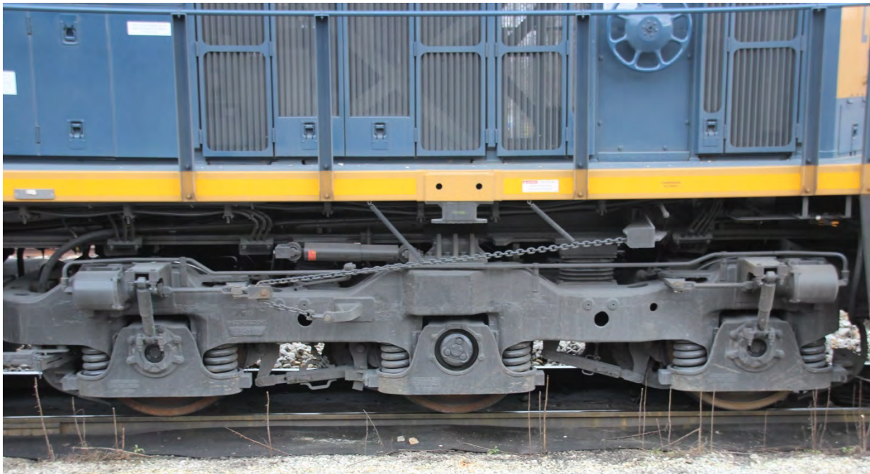
A close-up of the rear truck on CSXT 3318 showing the A1A wheel arrangement
