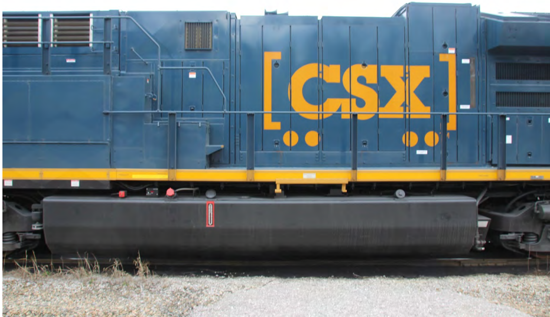
The middle left section of CSXT 3318 showing the fuel tank
