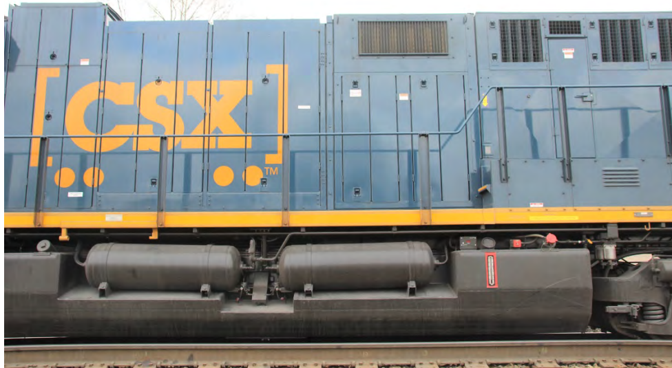
The mid-section of the right side of CSXT 3318 showing fuel tank and air reservoirs
