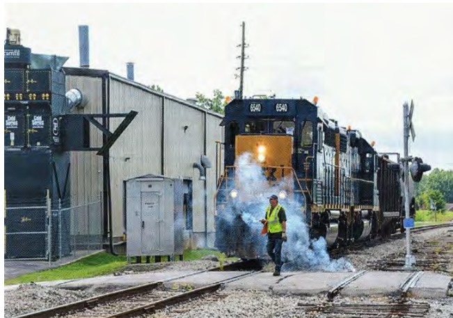
CSXT 6540 and CSXT 2524 were the power for the first run to Northwest Ordinance Distilling. Local Y128, which originated at Louisville's Osborn Yard, had in its consist an empty gondola for loading with ties and a loaded tank car for the plant. Note the fuzee burning on the crossing and the conductor talking the train over the road. (Lee Gordon)
