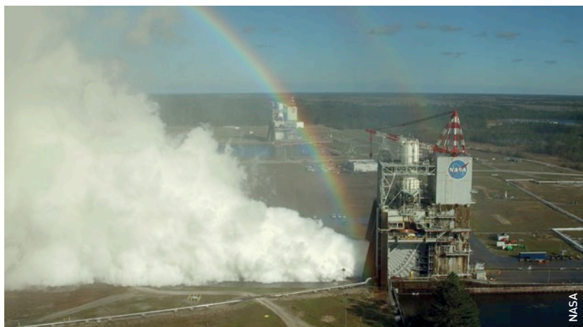
▲ The SLS programme and prime contractor Aerojet Rocketdyne have been testing new engine controller units for the RS-25 main engines at NASA's Stennis Space Center in Bay St Louis, Mississippi. The engines are also being certified to ensure they can withstand the increased propellant pressure and temperature inlet conditions they will experience during the first flight of SLS and Orion.
