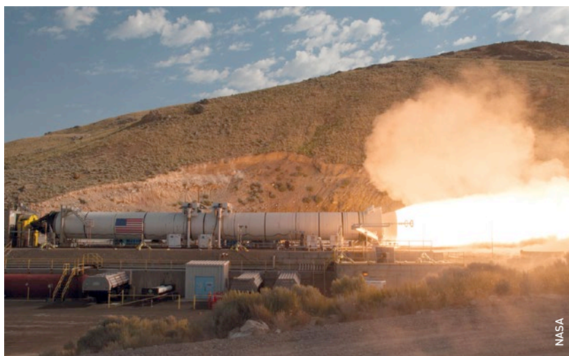
▲ The solid rocket motors that SLS uses have five propellant segments compared to the four-segment motors for the Space Shuttle. NASA and prime contractor Orbital ATK have conducted several static tests of development and qualification motors as part of the flight certification process.
