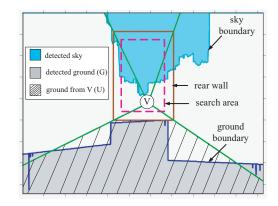
Figure 6: Determination of the best vanishing point.
