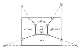
Figure 5: The partition of an image for a cuboid model. An image is partitioned into five areas, corresponding to the five faces of a cuboid model, rear wall, right wall, left wall, ceiling and floor.
