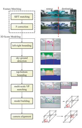
Figure 3: 3D scene model reconstruction.
