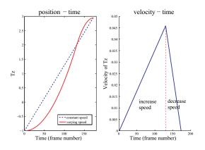
Figure 7: Examples of speed control functions.
