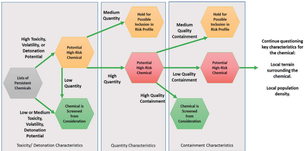
Figure 7. Example HID for identifying potential chemical hazards.
