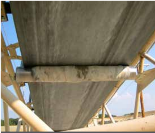
BUILD-UP CAUSES BELT MISTRACKING
