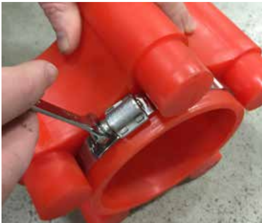
STANDARD HOSE CLAMP SECURES DISC
