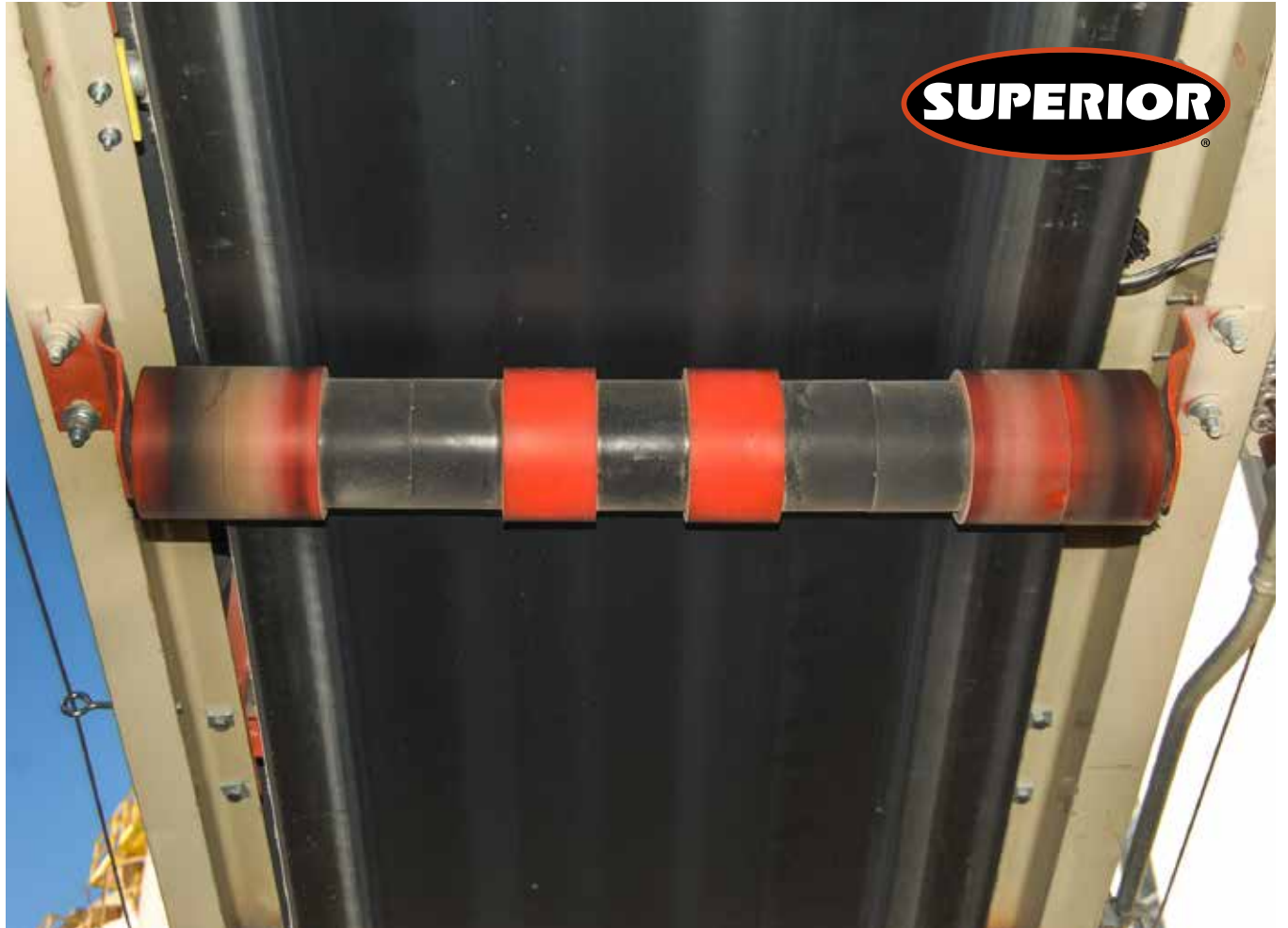
BUILD-UP CAUSES BELT MISTRACKING
