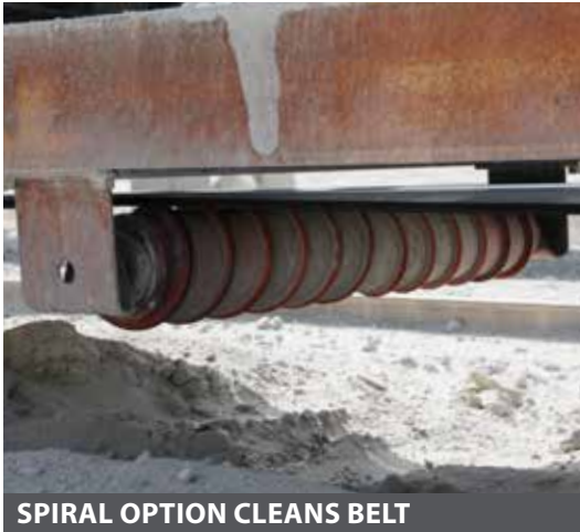
BUILD-UP CAUSES BELT MISTRACKING
