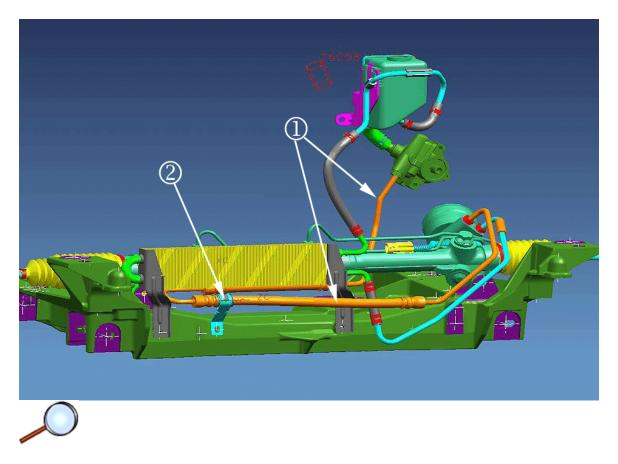
For vehicles with either FE3 or FE4 suspension, a screw, P/N 11609268, is also required. After installing the new hose (1), secure the clip (2) to the front crossmember with the screw.
