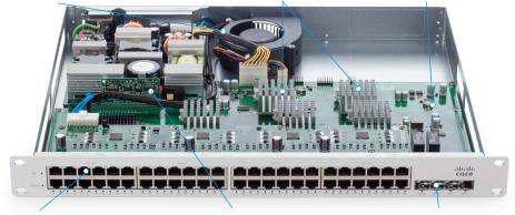
48× 1 GbE Ports with 802.3af/802.3at PoE/PoE+ Enhanced CPU / Memory Meraki Cloud Management Built-in 4× 10 GbE SFP+ Ports for Core Connectivity / Stacking
