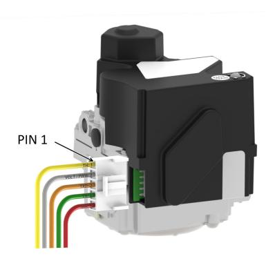
**Harness Interface:** JST 5-pin connector S5P – VH or equivalent with the following pin out configuration (mating connector VHR-5N). Use PIN SVH-21T-P1122-18AWG, or PIN SVH-41T-P1120-16AWG
