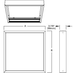
Regress Panel Field Assembly Luminaire
