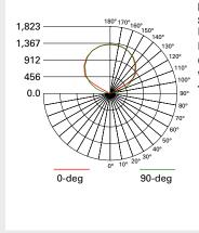
FILE NAME: S122IW-S675U835-4F0-1E-UDD LUMENS: 6803.6 Lms LPW: 129.3 LPW CCT: 3500K WATTS: 52.6 W TEST NUMBER: P331537
