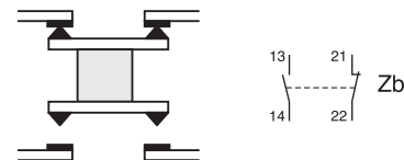
The 2 moving contacts are electrically separated
