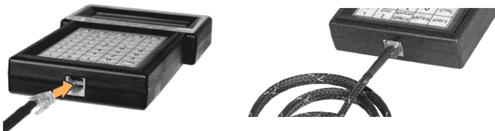
Figure 2-5. CA-0020526 RJ-11 Connector to CLC-10 Connection
