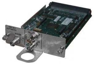
Figure C-1. CDI-10-1 Single G.703 (E3/T3/STS-1) Data Interface Module
