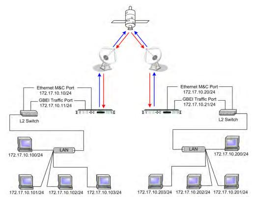
Figure E-5. CDI-70 GBEI Example: Bridging Remote Host on Common LAN over Satellite
