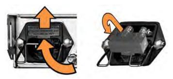
Figure 4-6. Replace the AC Fuses
