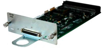
Figure D-1. CDI-60 HSSI Data Interface Module
