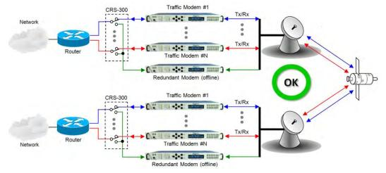
Figure A-5. Wired-thru for Hub-to-Hub with Standard Traffic using Routers
