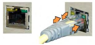
Figure 4-3. RJ-45/RJ-48 Connector Example
