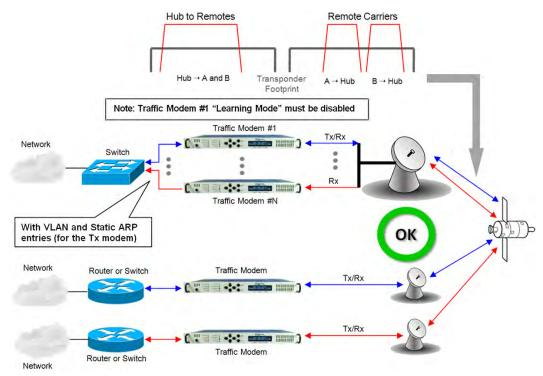
Figure A-13. Point-to-Multipoint using Switches
