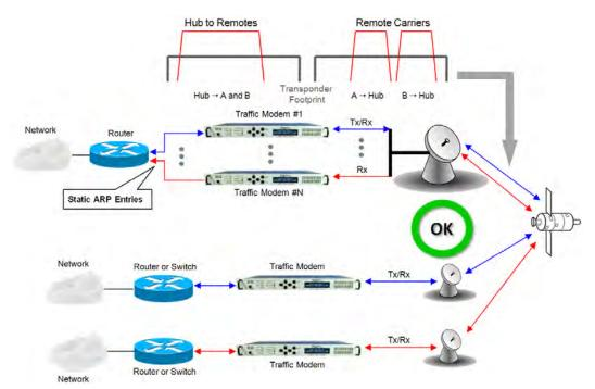
Figure A-10. Point-to-Multipoint using Routers
