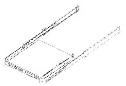
Figure 3-4. Install the Optional Rack Slide Set
