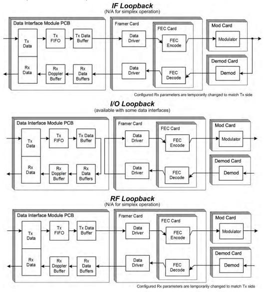
Figure 7-2. Traffic Data Flow Diagrams – Loopback Test Mode Examples
