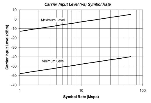
Figure 2-2. Demodulator Input Level
