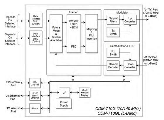
Figure 1-3. CDM-710G/L Block Diagram
