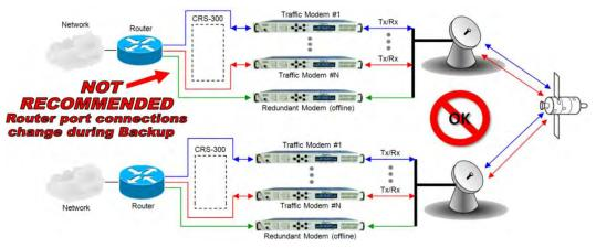
Figure A-6. Wired-around for Hub-to-Hub with Standard Traffic using Routers
