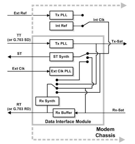
Figure F-2. Typical Data Interface Diagram (Features Vary By Interface)
