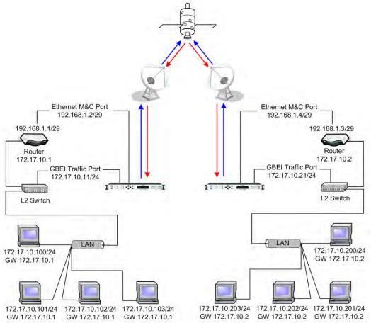
Figure E-6. M&C Port Assignment Example: IP Address NOT on Common LAN
