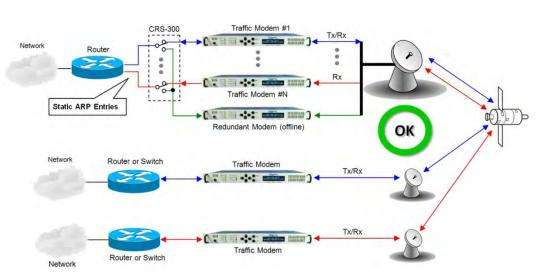
Figure A-11. Wired-thru for Point-to-Multipoint with Routers
