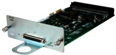
Figure F-5. CDI-60 HSSI Data Interface Module
