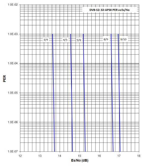
Figure B-4. DVB-S2 32APSK Packet Error Rate versus Es/No
