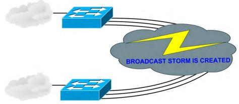
Figure A-3. Networking Loop Example (Simplified)
