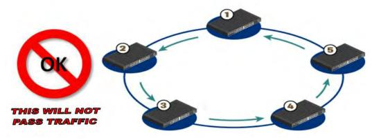
Figure A-1. Networking Loop with Switches
