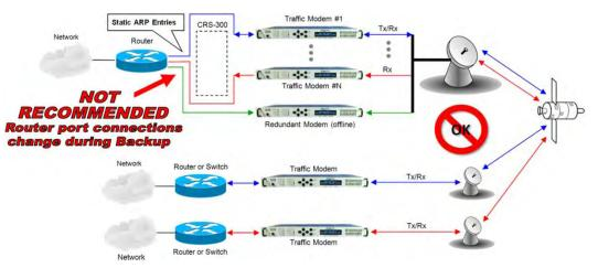
Figure A-12. Wired-around for Point-to-Multipoint with Routers
