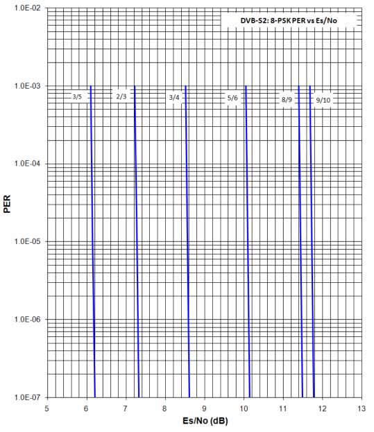
Figure B-2. DVB-S2 8PSK Packet Error Rate versus Es/No
