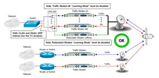
Figure A-14. Wired-thru, Hub-to-Remotes, Split-path Traffic using Switches (Point-to-Multipoint)
