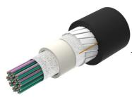
Fiber indoor/outdoor cable, All-Dielectric, LSZH Riser-Rated, Gel-Free, Central Tube Rollable Ribbon, 432 fiber, Singlemode G.657.A2/B2, Feet jacket marking, Black jacket color, Cca flame rating
