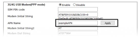
This will move the APN Name into the **Modem Initial String** to indicate that it has been saved.
