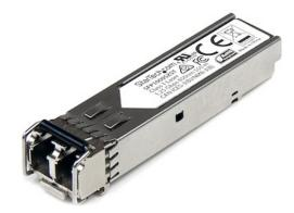
The SFP1000SXST is an MSA compliant fiber SFP transceiver that's designed, programmed and tested to work with 1000BASE-SX compatible MSA switches and routers. The SFP transceiver module supports a maximum distance of up to 550 m (1804 ft) and delivers dependable 1 GbE connectivity over fiber cabling. <br/> <br/
