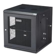
This 12U server or network rack cabinet lets you mount your EIA-310 compliant equipment to the wall, in a secure enclosure that has a hinged rear door for easy access to your equipment. The enclosure features adjustable mounting depth from 2.4 to 19.7 in. to provide a robust storage solution for your rack-mount equipment.
