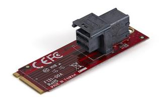
This PCI Express U.2 to M.2 adapter makes it easy to install a high-performance U.2 PCIe-NVMe SSD into your desktop PC or server and connect the drive through an M.2 PCIe x4 slot on your motherboard. By creating compatibility with newer U.2 NVMe SSDs, such as the Intel SSD 750 series, this enterprise-class drive adapter enables you to gain faster read/write speeds and higher productivity levels for data-intensive applications.
