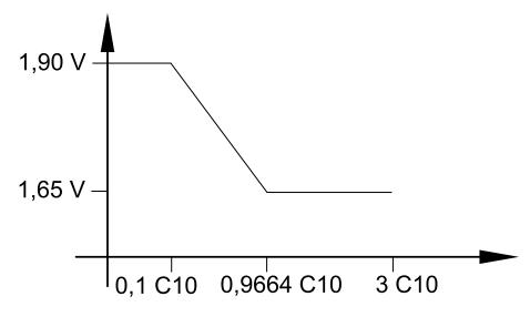
Shutdown voltage level versus the discharge rate/cell.
