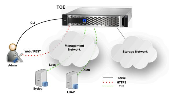
Figure 2: TOE Deployment
