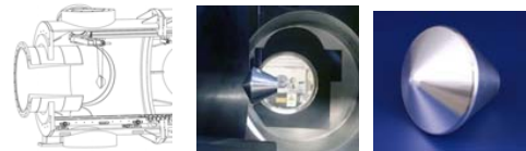
Fig. 1 Schematic (left) and photograph (middle) of the model setup in HEG; photograph of the model (right).
