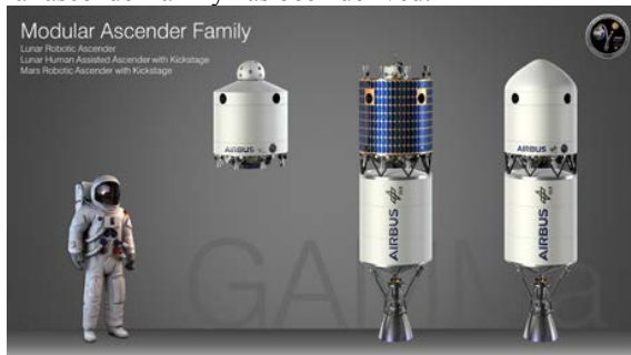
Fig.1: left: GAMMa LPSR ascender, center: GAMMa HERACLES ascender with kick-stage right: GAMMa MSR ascender with kick-stage
