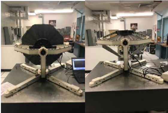
Figure 4. System-level accelerometer calibration on optical bench.
