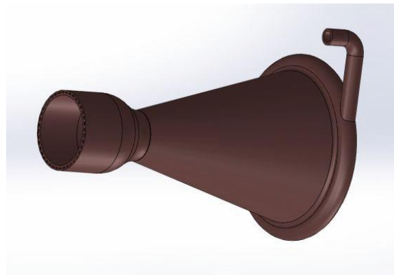
Figure 1. Nozzle and combustion chamber geometry.
