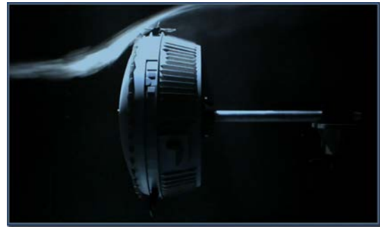
Figure 2: Photograph of the Huygens mock-up under test: flow visualisation
