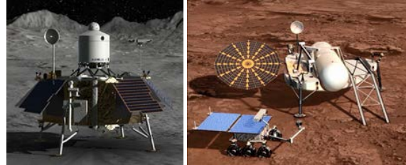
Fig.1: left: GAMMa LPSR lander, right: GAMMa MSR lander with sample fetch rover
