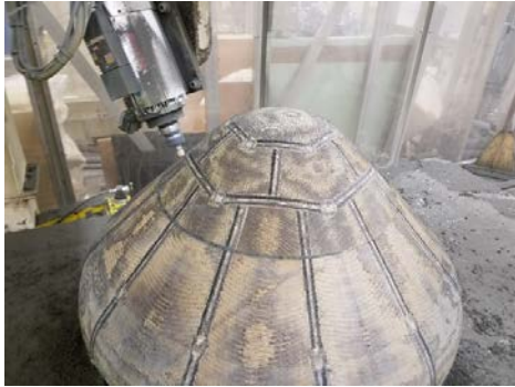
Figure 2. 3-D Woven dual-layer heat-shield (HEEET) undergoing outer mold line machining.
