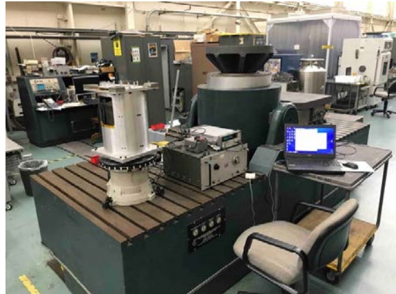
Figure 5. System-level rate gyro calibration on spin table.
