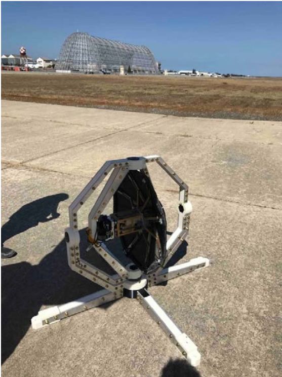
Figure 3. Magnetometer calibration at Moffett Field compass rose
