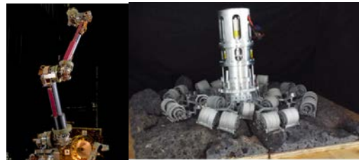
Figure 2. 7-DOF robotic arm and Microspine Gripper
