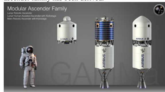
Fig.2: left: GAMMa LPSR ascender, center: GAMMa HERACLES ascender with kick-stage right: GAMMa MSR ascender with kick-stage
