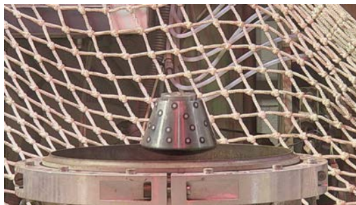
Fig 1. A capsule shaped test model free-flying in the test section of the vertical wind tunnel DLR-VMK.
