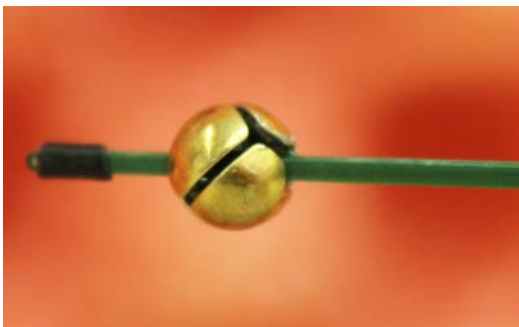
Fig. 1. Photograph of the prototype of the spherical sensor anemometer.
