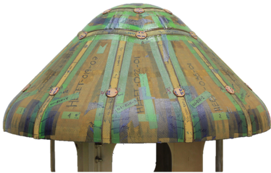
Figure 1: HEEET ETU Before OML Machining
