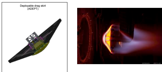
Figure 3. A deployable skirt concept made of 3-D woven carbon fabric can withstand the heating and based on ADEPT studies, the foldable construct could be an option if launch constraints require the deployable skirt to be folded during launch.
