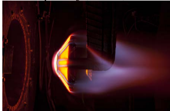
Figure 1: High-definition video capture of the ADEPT arc jet article in the Interaction Heating Facility (IHF) at NASA Ames Research Center.
