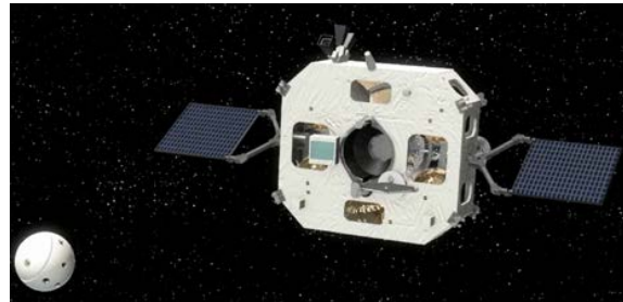
Fig.2: Free flying capture of orbiting sample (MSR, LPSR)
