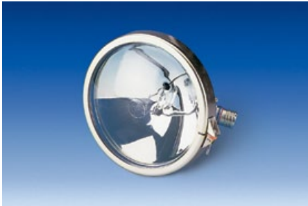
Nose Gear Landing Light 1X0455068-02
